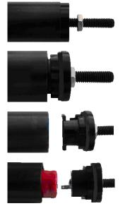
6.1.5 Slightly pull out the PCB board tills the SIM Card slot shows up.
