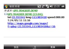
**\*Tracking location** When no GPS signal, the SMS includes the last valid latitude & longitude as well as the LAC code of current position, the LAC code can be input in the column of "manual track" menu of web platform to check location.
