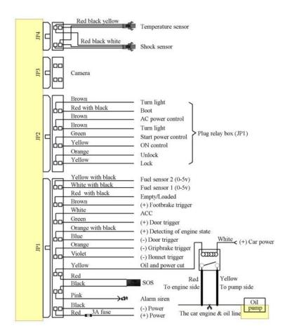
\*Orange with black wire of JP1: Engine status detection, it is used to detect the engine started or not after automatically start command, this wire connects to the power wire of fuel pump(for gasoline vehicle) or output wire of generator (for diesel vehicle), and
